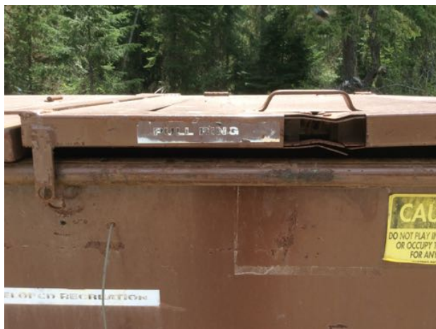
Photo 9: White Sand Campground—this dumpster’s safety features are no longer functional. A bear could push up the lid and crawl in.
